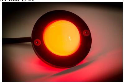
Comprising an aluminium structure, Conduit LED is an attractive versatile light source. Each unit integrates Single colour, RGB, RGBW or blue / white LEDs. The LEDs are combined with control electronics to form a compact high output light unit which is compatible with metal and plastic 20mm conduit fittings. An optional adjustable eye lid makes the system ideal for stair / floor way lighting.
